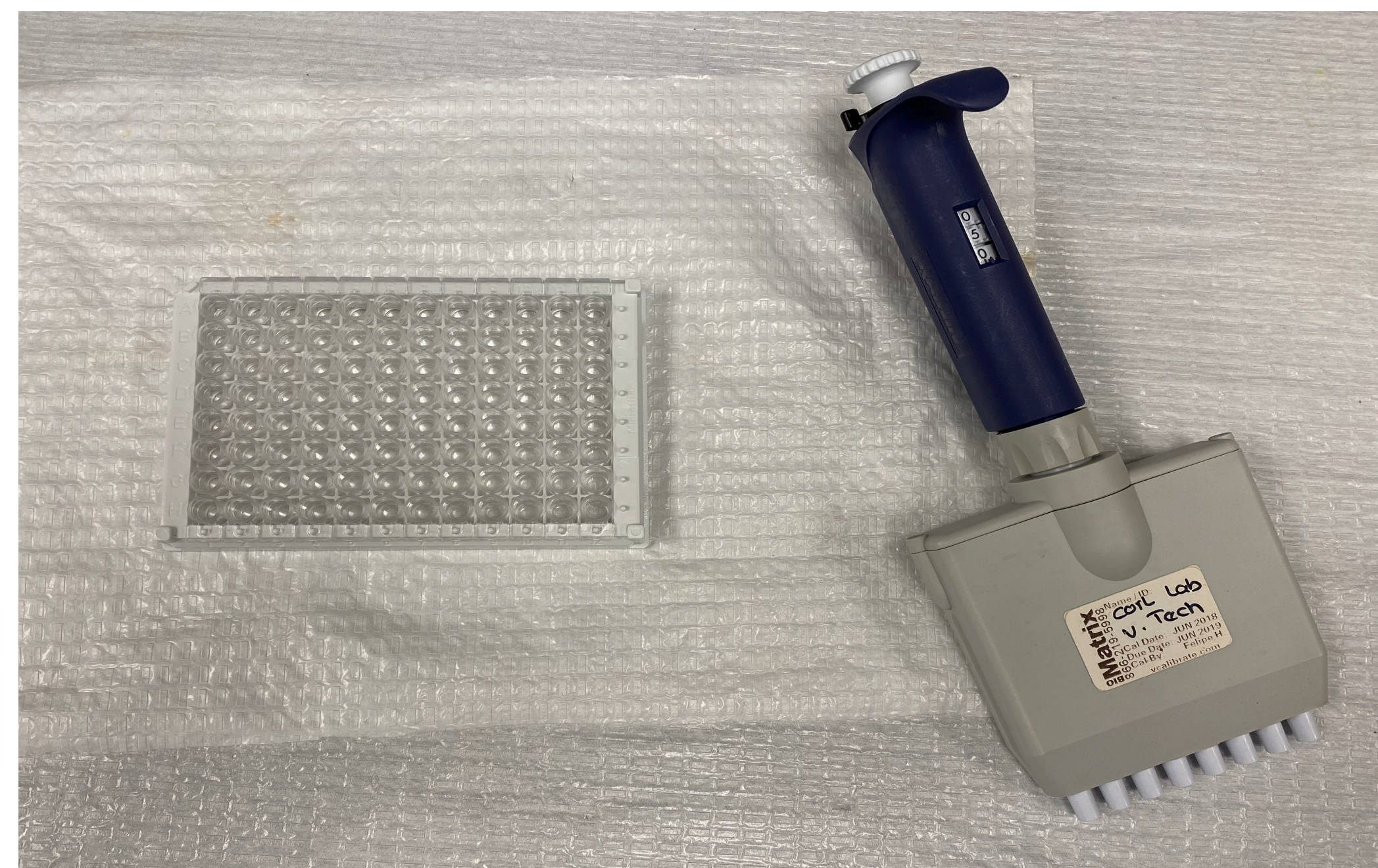
Figure 2: 96 well plate for plate reader assay and Multi-Channel Pipette
