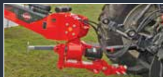
Standard drawbar or 2-point Gyrodine® swivel hitch for tight turns
